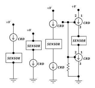
By using a CRD to bias your sensors, it is possible to reduce the noise and increase the accuracy of your sensor, especially in a noisy electrical environment. The CRD will also act as an Analog Switch.
