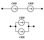
The Current Regulator Diodes (CRDs) will evenly split the load across multiple devices to increase the Voltage or Current carrying capability. By adding CRDs in series and parallel both the current carrying, and the breakdown voltage capability can be increased.
