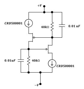
This Cascode floating current source will regulate **15-30V** to **0.00005%/V** supplying **200uA**. The output impedance will appear to be **10** G $\Omega$ . The low voltage compliance is limited by the combination of the gate reference voltages to around **8V**. The high voltage compliance is limited by the lower voltage rated JFET.
